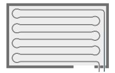
Pipe is laid in parallel runs up and down the room length, with loop turns at each end. Hep<sub>2</sub>O panel products all use the serpentine pattern and it can also be used with staples.
