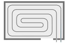
Initially at 400mm centres this layout follows the room shape in a spiral to the middle and is then reversed out from middle. This leaves pipe spacing at 200mm centres. This pattern is possible with two Hep<sub>2</sub>O underfloor heating systems - Staples and System Plates. With spiral patterns, close centres can generally be achieved without excessively tight turns.
